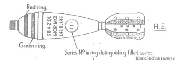
Weight 9.1kg (20lbs) Firing Mechanism Trip (small trigger)
