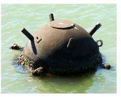
Buoyant mines, designed to drift free, float or sit just below the surface, were the most commonly deployed marine mines. They were typically moored, or tethered to the seabed with an anchor or wire.
