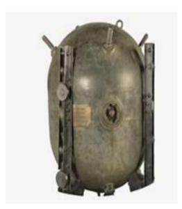
German ground mines (Luftmine) were air-deployed naval mines which were also modified for deployment from submarines and surface craft. Although primarily designed to lie on the seabed, many were also moored or buoyant. Designed as an anti-shipping weapon, the WWII Luftmine was also often used on land based targets.
