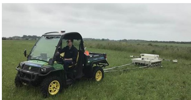
Example of a towed magnetometer survey platform
