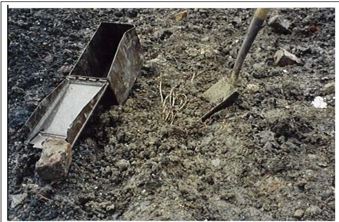
**Plate 2** Cordite Propellant In The Ground
