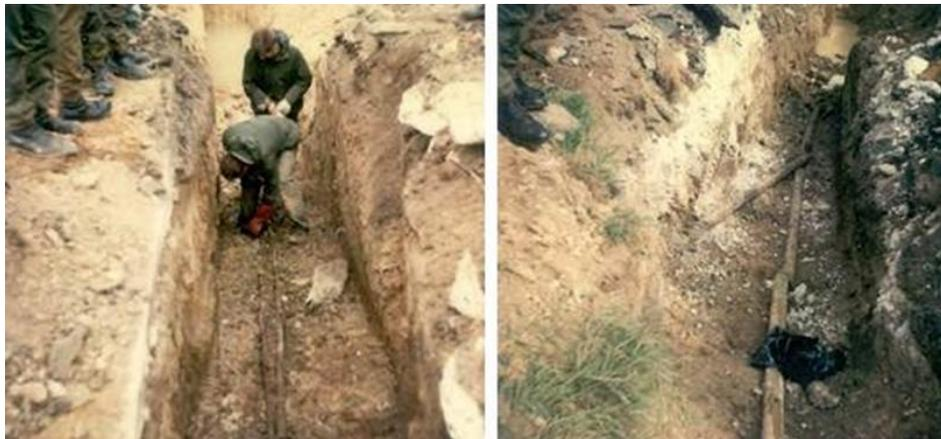
**Hazard** The investigation of pipe mines is undertaken with extreme caution due to the increased probability of an accidental detonation as a result of the instability of their Nitroglycerine content.
